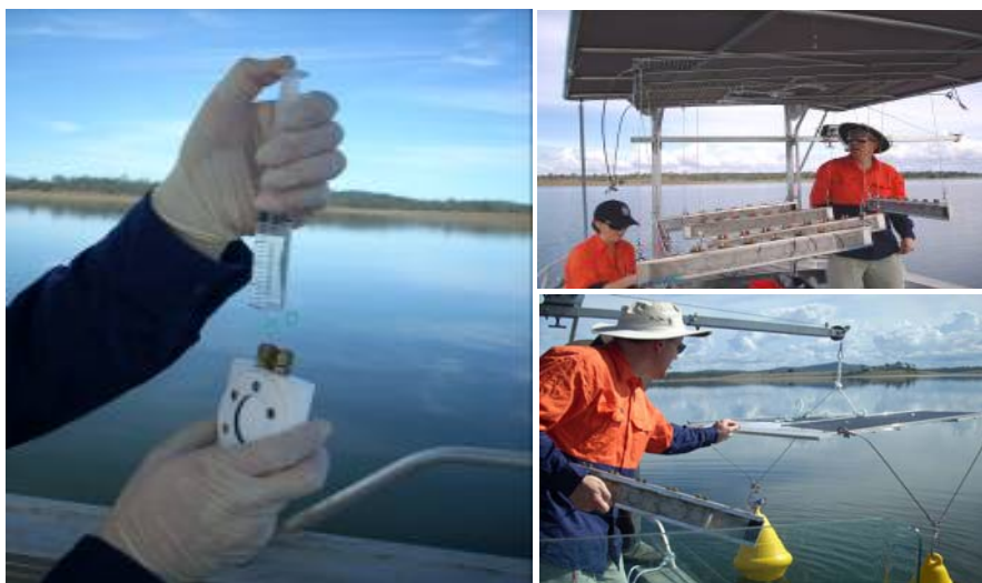
Figure 2. Set up of pathogen decay chambers in Lake Wivenhoe
