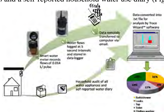
Figure 1. Schematic flow of process for acquisition, capture, transfer and analysis of water flow data.
