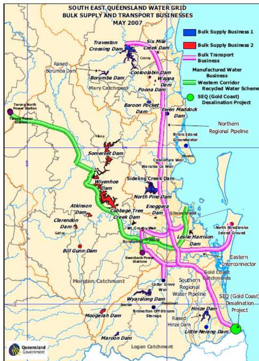
Figure 2 Schematic diagram of the South East Queensland (SEQ) Water Grid, which will include the WCRW project. (Urban Water Supply Arrangement in South East Queensland 2 )
