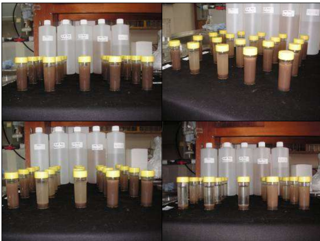
Figure 25: Samples of the four soils (rows) x five waters (columns) showing settling 4 minutes (top left), 10 minutes (top right), 1 hour (bottom left) and 22 hours (bottom right) after agitation.
