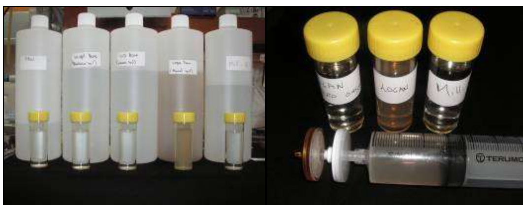
Figure 23: The five water qualities tested: five 1 litre bottles on left – PRW, Voigt bore, University of Queensland bore, Logan Dam and Milli-Q deionised; and three vials on right – clarified Logan Dam water after passing through a 0.45µm filter, unclarified Logan Dam and Milli-Q deionised water.
