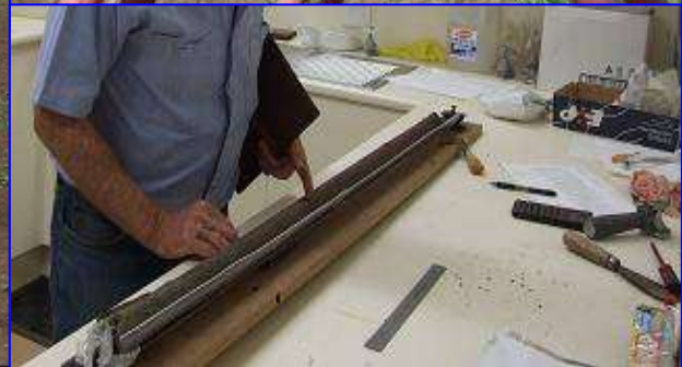
Photo 2: Removable PVC liners inside coring tubes.
