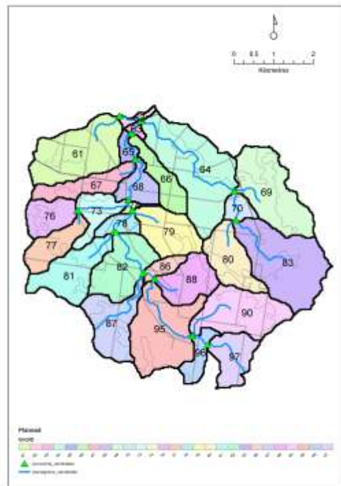
Figure 5. Cropped set of sub-catchments used for runoff modelling of the Ripley Valley (numbers are for sub-catchment ID, green triangles indicate sub-catchment pour points).
