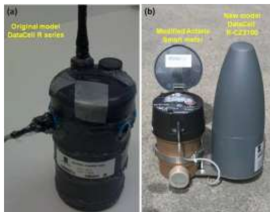
(a) Waterproofed logger. (b) Smart meter and new series data logger.
