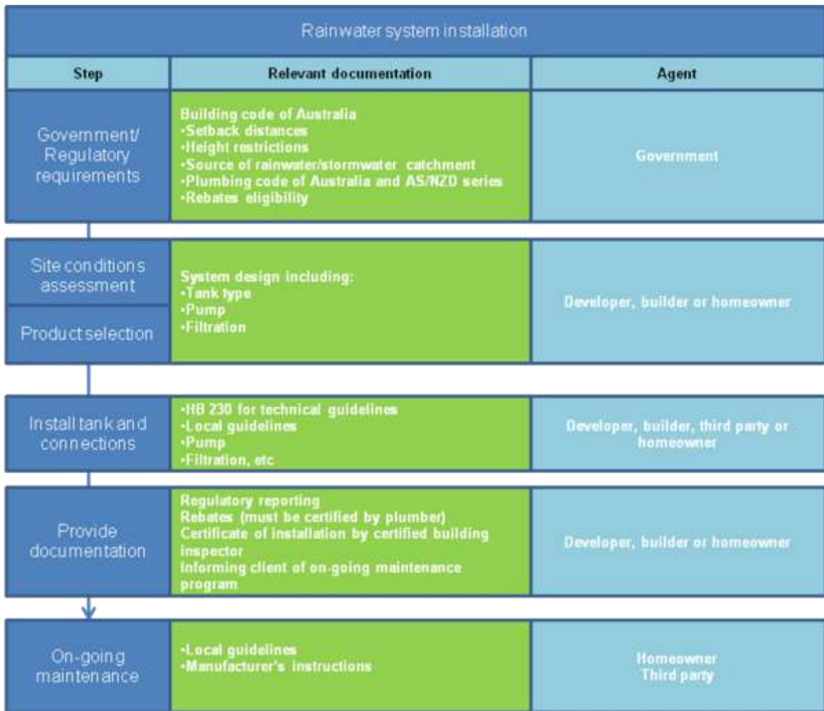
Figure 2. Process for installation of rainwater systems*.
