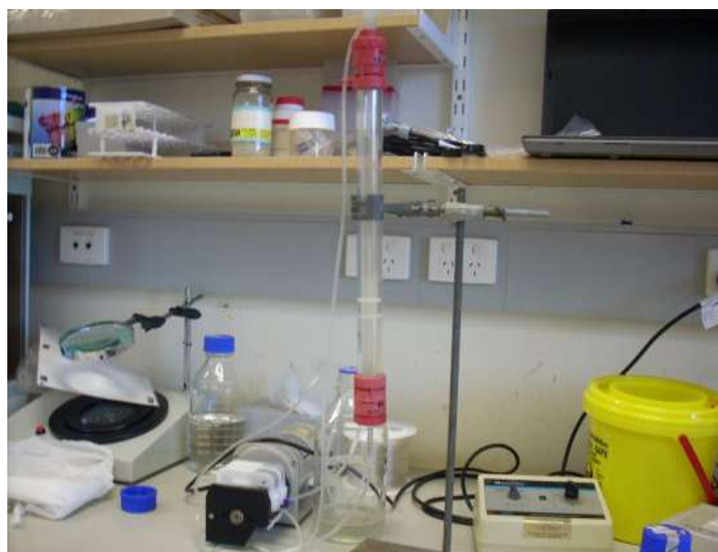
Figure 3. Modified chromatography column apparatus for virus concentration.
