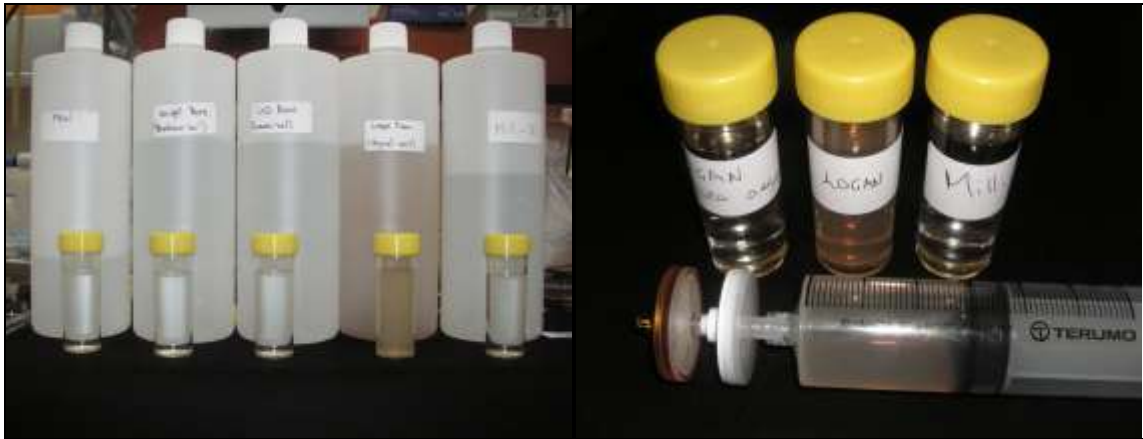
Figure 2: The five water qualities tested (from left to right – PRW, Voigt bore, University of Queensland bore, Logan Dam and Milli-Q deionised); and clarified Logan Dam water after passing through a 0.45µm filter (right).
