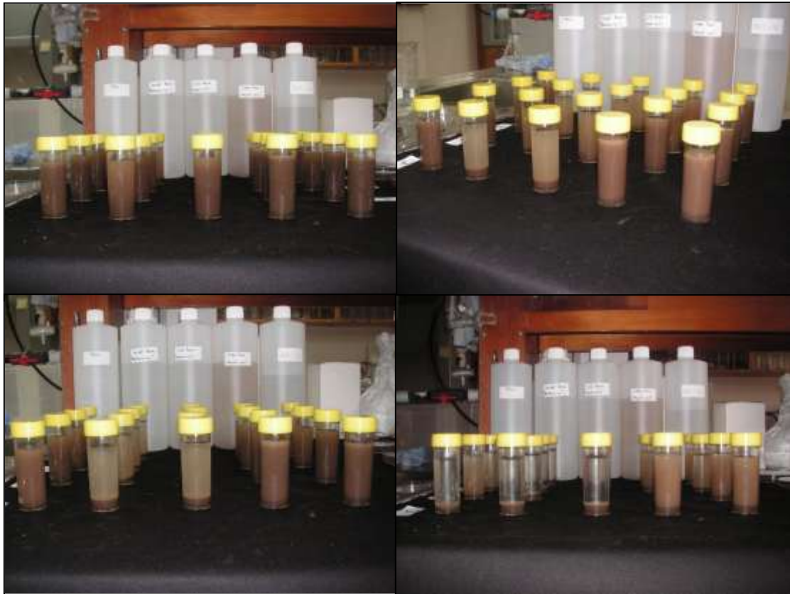
Figure 4: Samples of the four soils (rows) x five waters (columns) showing settling four minutes (top left), 10 minutes (top right), one hour (bottom left) and 22 hours (bottom right) after agitation.
