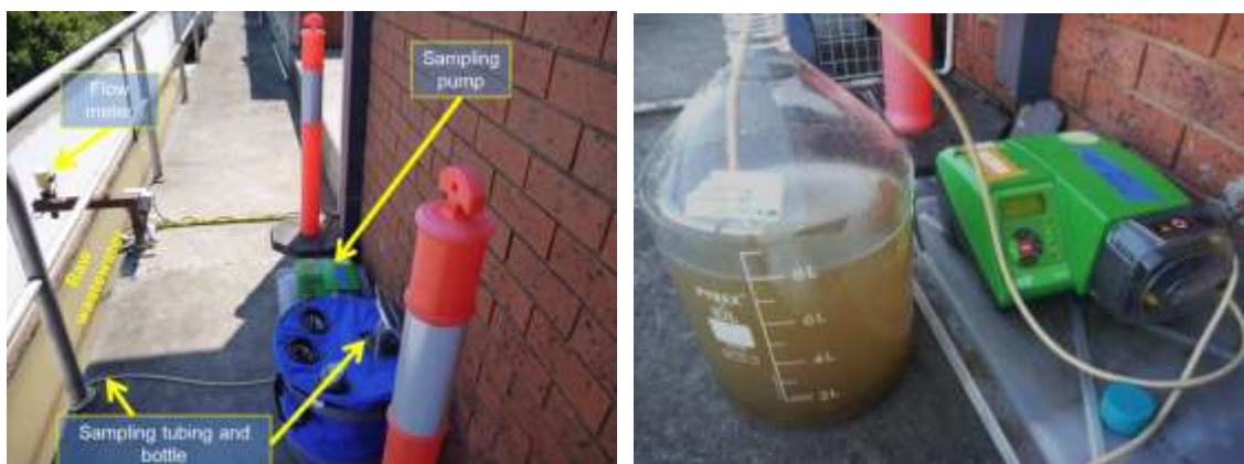
Figure 13. Flow proportional sampling set up at Bundamba STP and sampling bottle after a 24h cycle.
