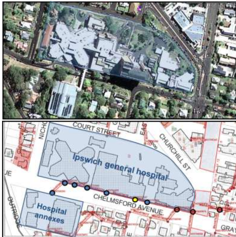
Figure 8. Aerial view of Ipswich Hospital and its corresponding sewerage network map. (The blue dots correspond to sewers exclusively collecting hospital wastewater, the reds dots to sewers collecting hospital wastewater along with domestic wastewater from households nearby and the yellow dot the sewer chosen for sampling).
