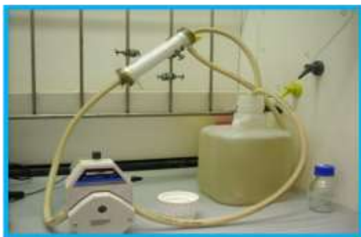
Figure 4. Concentration of water samples using hollow fibre ultrafiltration cartridge, shown in the top of photo. The raw water sample is in the container on the right. A peristaltic pump (bottom left) supplies pressure to pass the water through the UF cartridge.
