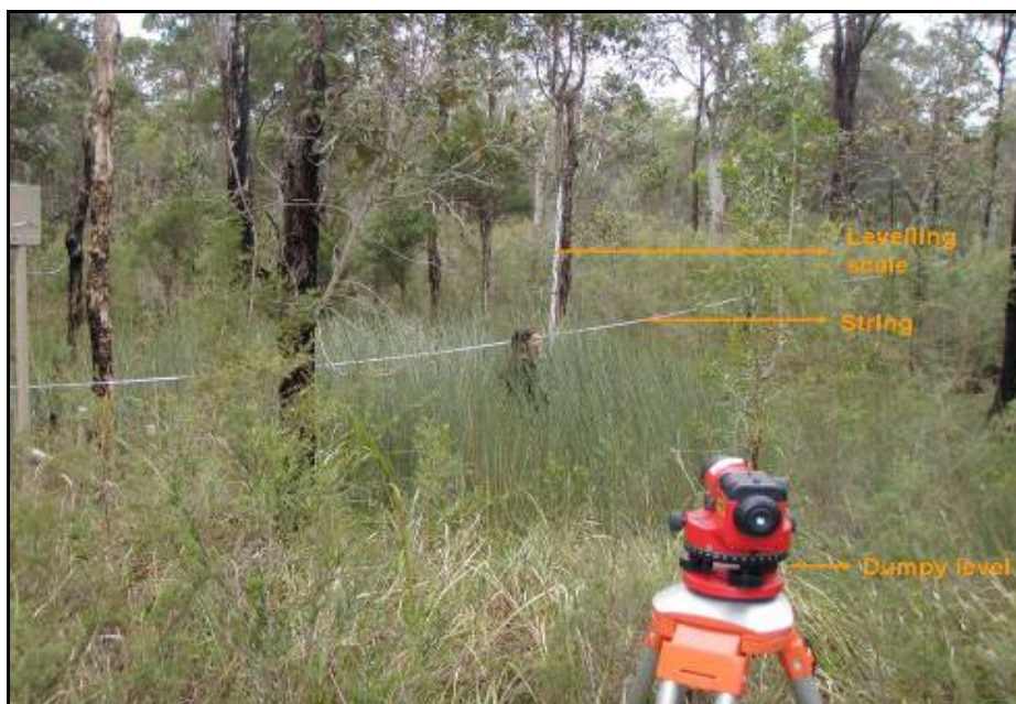
Figure 18: Surveying the cross section of the gauging location at Scrubby Creek, Karawatha Forest using a Dumpy level.
