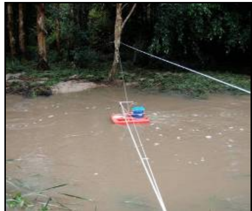
Figure 22: Low and medium flow gauging using a current meter (left) and high flow gauging using an Acoustic Doppler (right).
