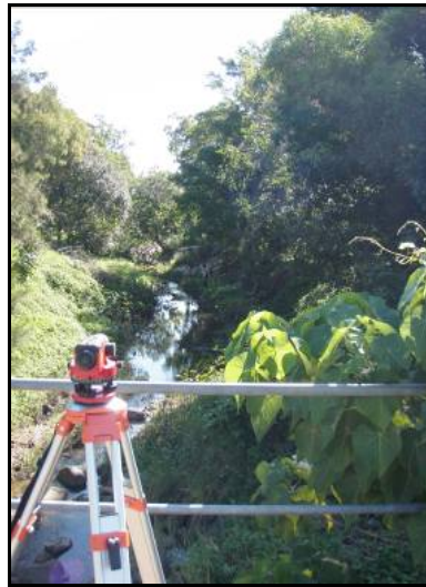
Figure 20: Surveying water surface slope at Stable Swamp Creek, Sunnybank using pegs installed during a prior high flow event.
