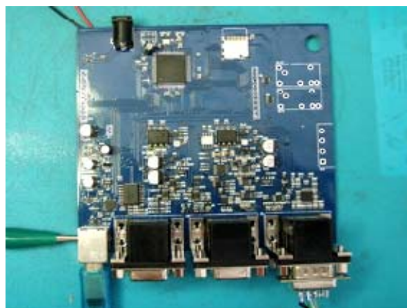
Figure 16. The 1st generation integrated sensor control electronics with on-board computer.
