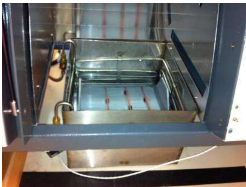
Figure 26. Overview of internal set-up of Solar Simulator, with cuvettes submerged and fixed in place within the temperature-controlled water bath.
