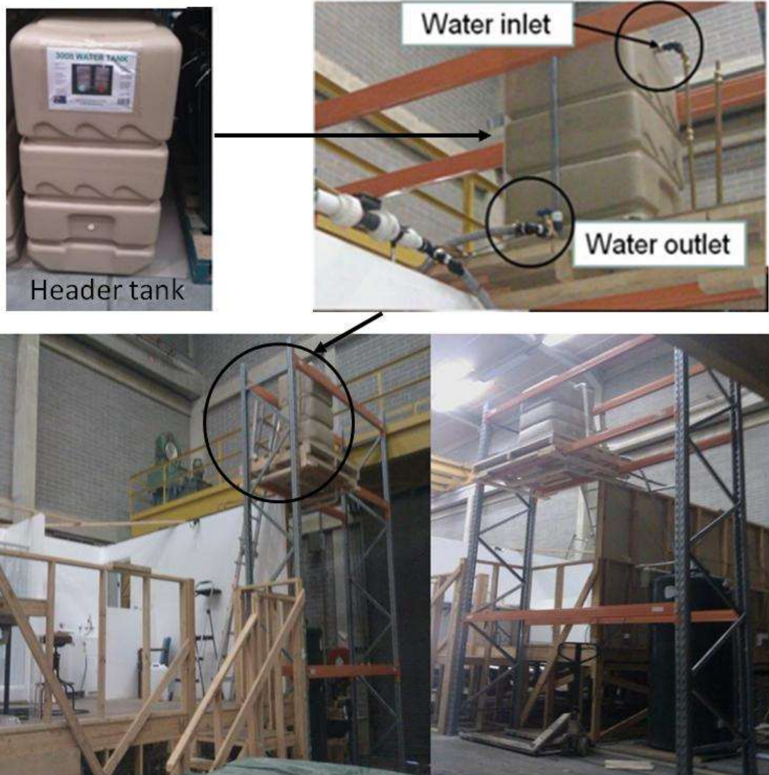
Figure 11: 300L header tank used in the analysis. It was located 2.7m above house floor level.
