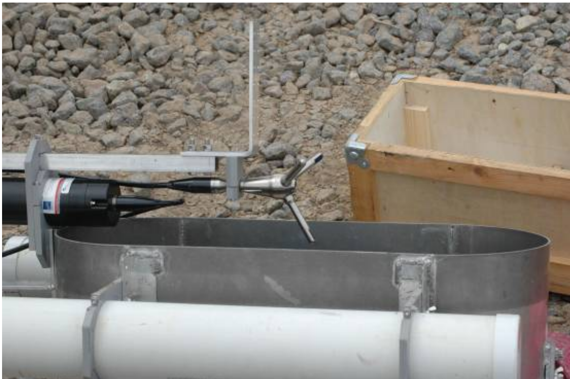
Figure 30: ADV mounting bracket allows vertical and horizontal adjustment of measurement volume.
