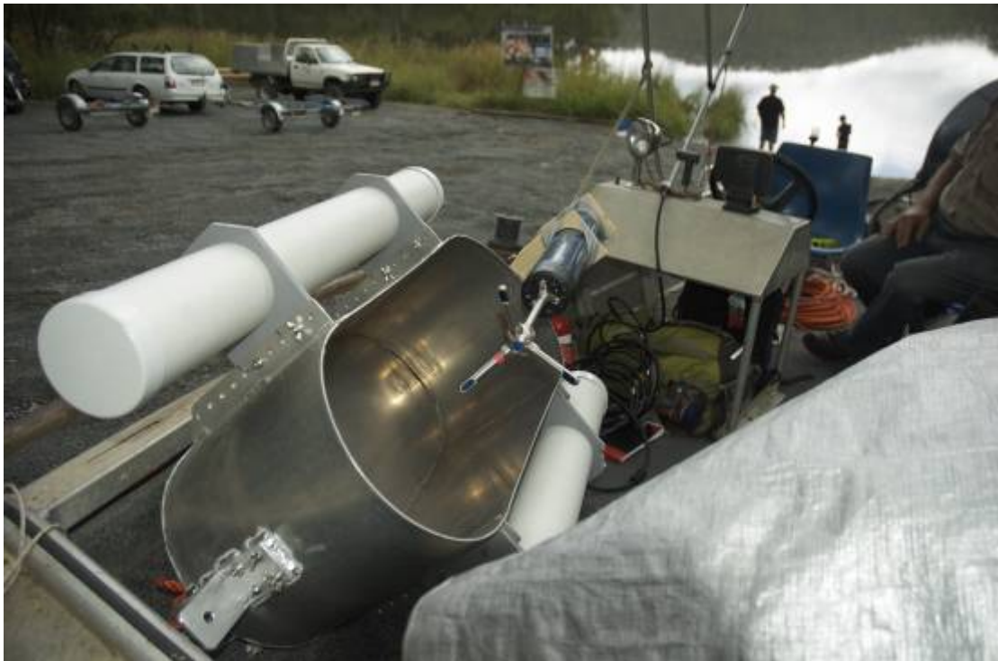
Figure 29: Photo of floating chamber with ADV attached using a temporary mounting bracket.
